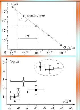
Fig 2. Theoretical estimations for lifetimes  $t_m$  of photo-integrated structures of second-order susceptibility  $\chi^{(2)}$  in isotropic media with dependent electrical conductivities  $\sigma$ .
