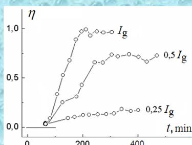
**Figure 3.** The dependence of the amplification of the photo-integrated initial lattices of the second-order susceptibility  $\chi^{(2)}$  during it's illumination by outside YAG:Nd laser 2 radiation  $d_{2\omega}$  with different intensities. The maximal pulse power for  $d_{2\omega}$  beam was  $P_{2\omega} \approx 40$  mJ, the maximal intensity for this radiation in focal place, correspondingly, was  $I_g \sim 10^9$  W/cm<sup>2</sup>.
