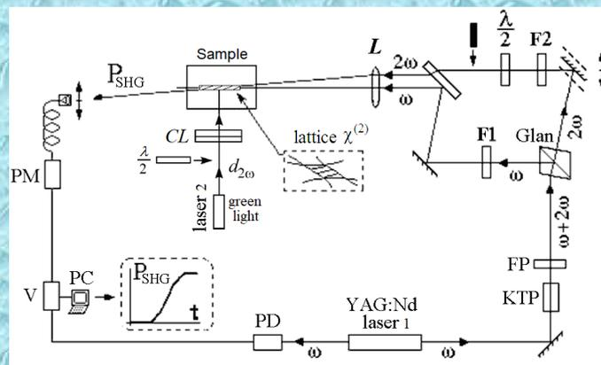
**Figure 2.** The scheme of the experimental set-up for OP and study of the outside green light stimulation of the photo-integrated micro-periodic second-order susceptibility lattices.
