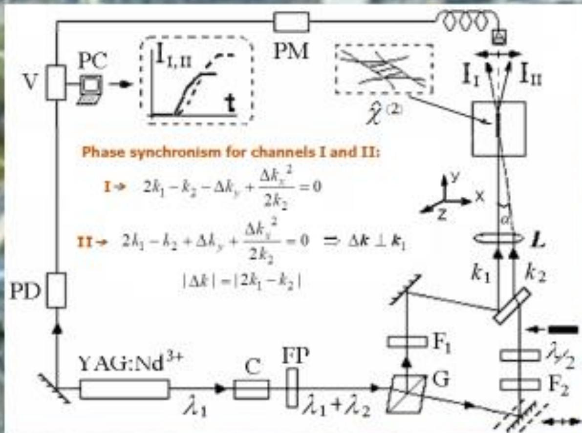
Experimental set-up for investigations of per-channel nonlinear-frequency conversion in volumetric all-optical poling
