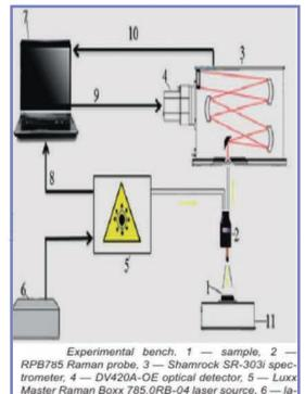
Master Raman Boxx 785.0RB-04 laser source, 6 — laser power supply, 7 — computer, 8, 9, 10 — control cables, 11 — coordinate table.
