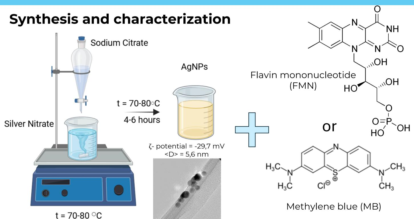
AgNPs demonstrated high colloidal stability and a local surface plasmon resonance (LSPR) peak at 435 nm. Citrate ions served as both the reducing agent and stabilizer for AgNPs.
